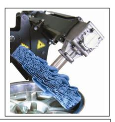
**2 – BRUSH FASTENING** - Choose suitable brush which will be used on the rim and fasten it to suitable parts.
