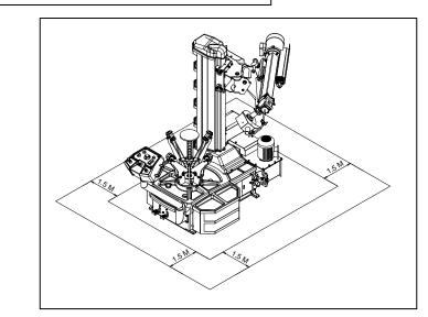
While the Machine is working or not working, Except the operator no one should not be close to the machine more than 1,5 meter distance and There should be at least 1,5 meter working area around the machine to provide the operator work comfortably.
