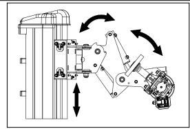
**CRADLE AND SUPPORT GROUP** During the Rim Polishing It provides to touch the brush easily whole surface of the rim.
