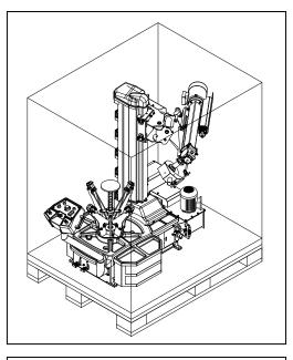
When you unpack the machine , please do check If the machine has got damaged or not during the transportation and please check If there is missing parts and equipment or not . During the unpacking Please pay attention to such as cutting materials Nail, Fiber, etc ....
