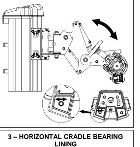
— Do push the joy stick which is showed on the figure to the right and left to make move Horizontal Cradle Bearing lining to down and up
