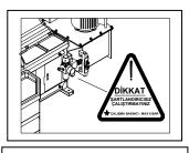
The operating pressure value is max. 8 bar.
